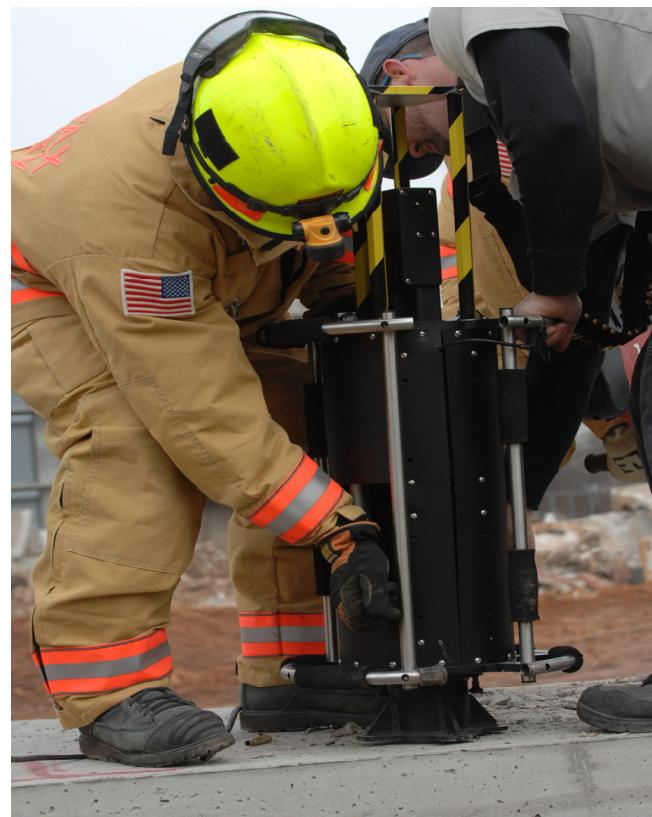
Firefighters test a CIRT prototype at a Fairfax, Virginia, facility. The device uses a blank ammunition cartridge designed for a standard hunting rifle—driving a piston—that, when fired, generates a high-energy jolt.
