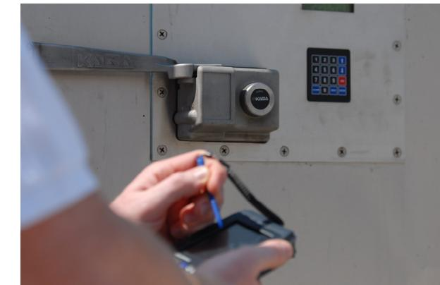
An electronic lock controls access to the milk tank and keeps track of when it is opened.
